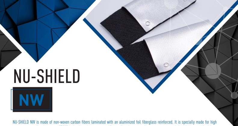
NU-SHIELD NW is made of non-woven carbon fibers laminated with an aluminized foil fiberglass reinforced. It is specially made for high temperature applications up to 250°C in harsh environments to reflect radiant heat away from components and the fabric material adds an insulating thermal protection layer.
