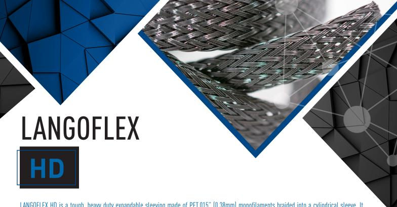
LANGOFLEX HD is a tough, heavy duty expandable sleeving made of PET.015" (0.38mm) monofilaments braided into a cylindrical sleeve. It provides excellent abrasion and good mechanical properties. The flexible open braid construction provides complete drainage preventing heat, condensation and moisture. The good chemical resistance of the polyester material makes it ideal for applications in harsh environments and in electronics, marine, and industrial wire harness applications.
