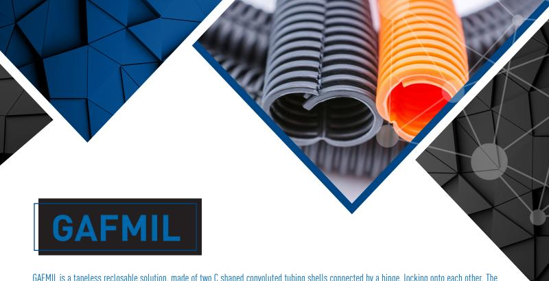
GAFMIL is a tapeless reclosable solution, made of two C shaped convoluted tubing shells connected by a hinge, locking onto each other. The first convolute portion takes place on the wire harness, the second portion pivots thanks to the hinge and covers the first one. The overlap between the two convoluted portions avoids the risk of wire exposure, even in low radius curve zones. This solution also allows an easy and quick installation on wires, while offering a filling ratio up to 100%.
